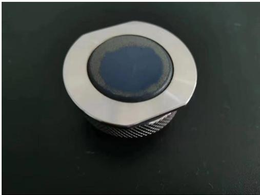
Photo 1 After wear resistance test for 600,000 times
